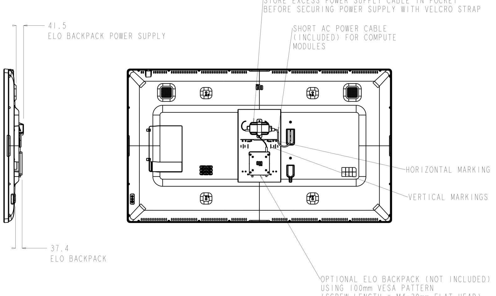
BRIGHTSIGN COMPUTE MODULE MOUNTING INSTRUCTIONS: I. ALIGN COMPUTE MODULE EDGE WITH HORIZONTAL MARKING 2. CENTER COMPUTE MODULE USING VERTICAL MARKINGS 3. INSTALL M4 SCREWS THROUGH DEVICE (MAX SCREW DEPTH INTO ET6554L = 5mm)
